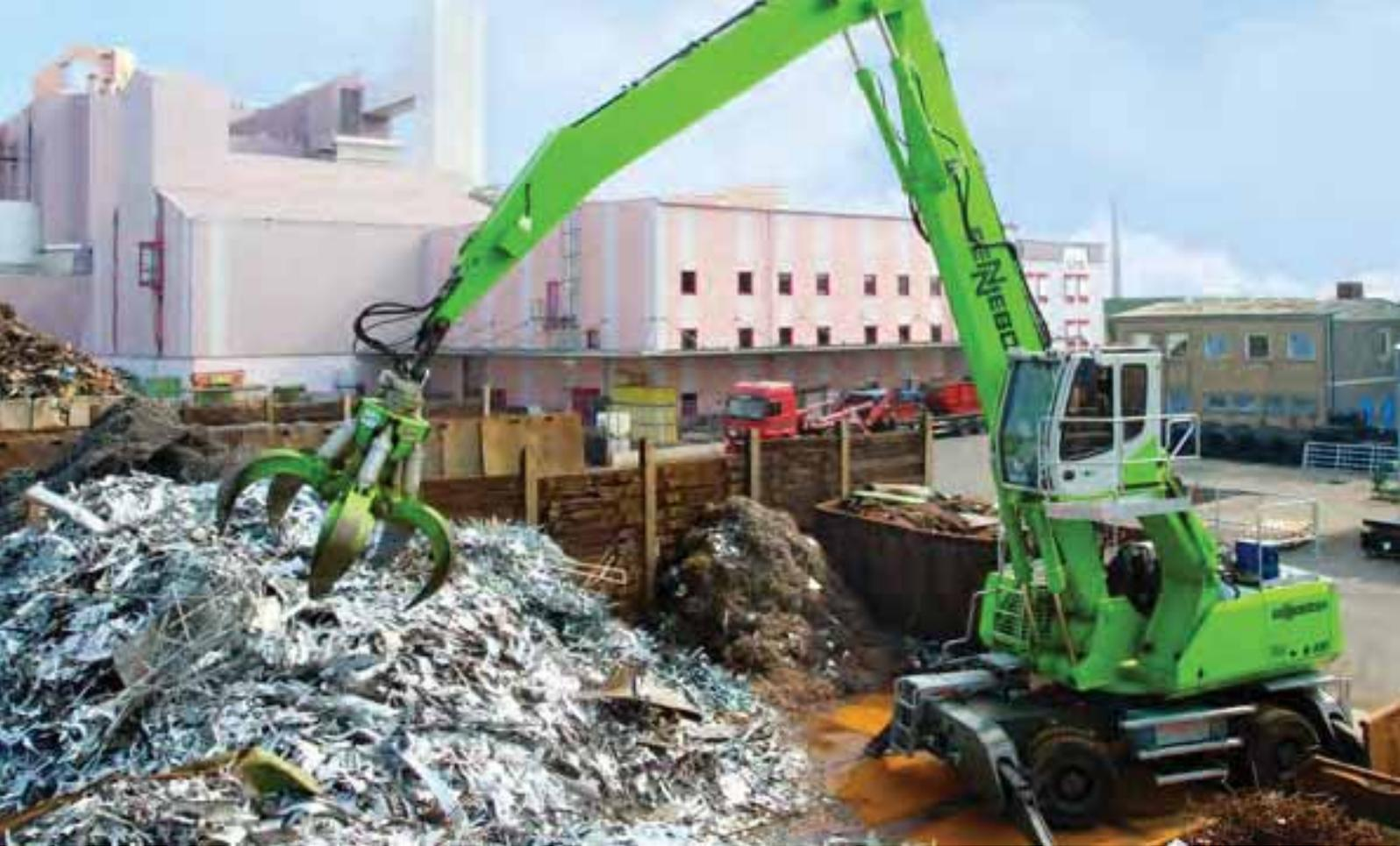
**830 M - with orange peel grab - feeding of a baling press with iron sheets; Germany**
