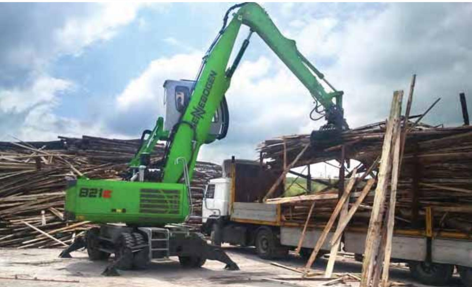
821 M - with sorting grab - unloading of used wood from truck; Russia
