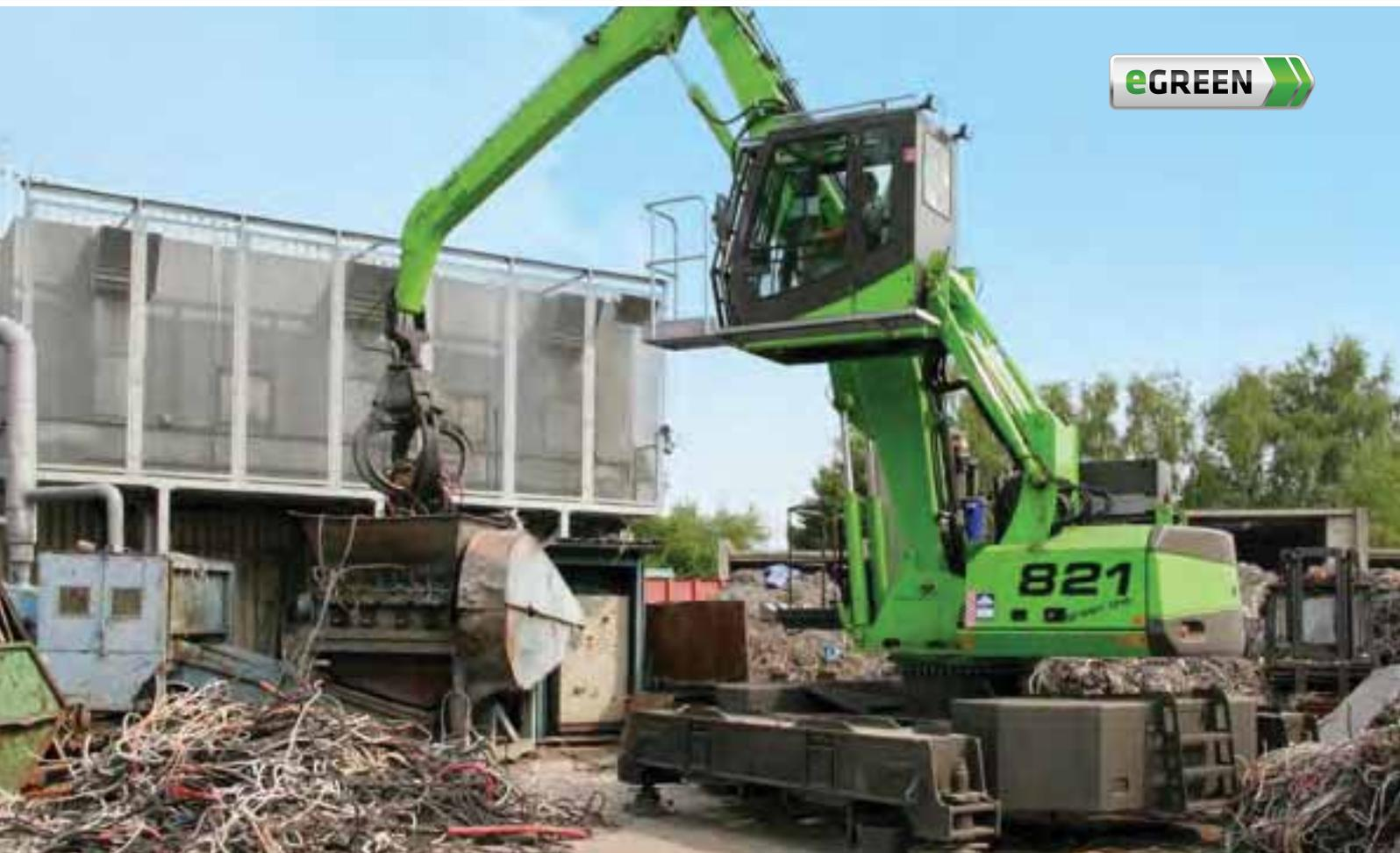
**821 stationary electro – with orange peel grab – feeding a shredder with electronic scrap; Germany**
