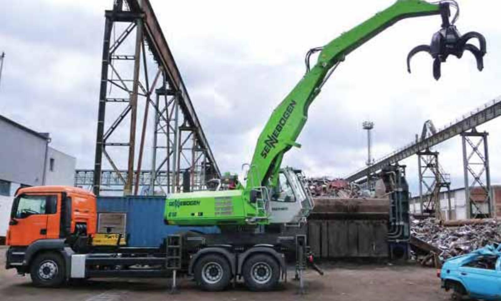
**818 truck mounted for fast changes of the job site – with orange peel grab – scrap recycling; Czech Republic**
