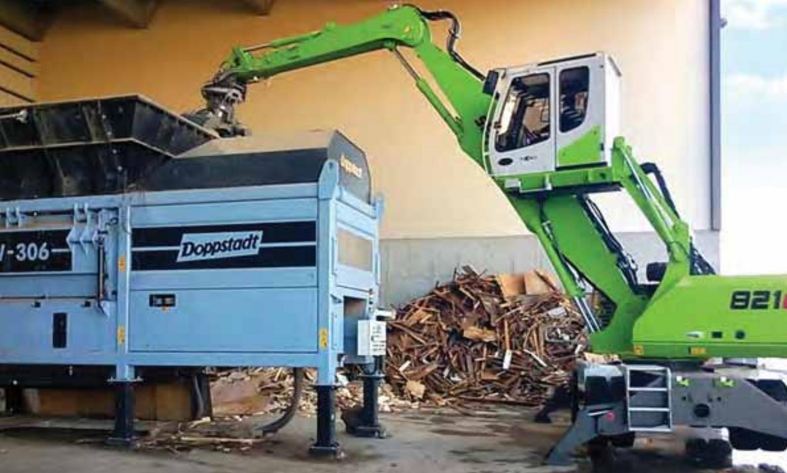
821 M – with sorting grab – feeding a shredder with used wood; Japan
