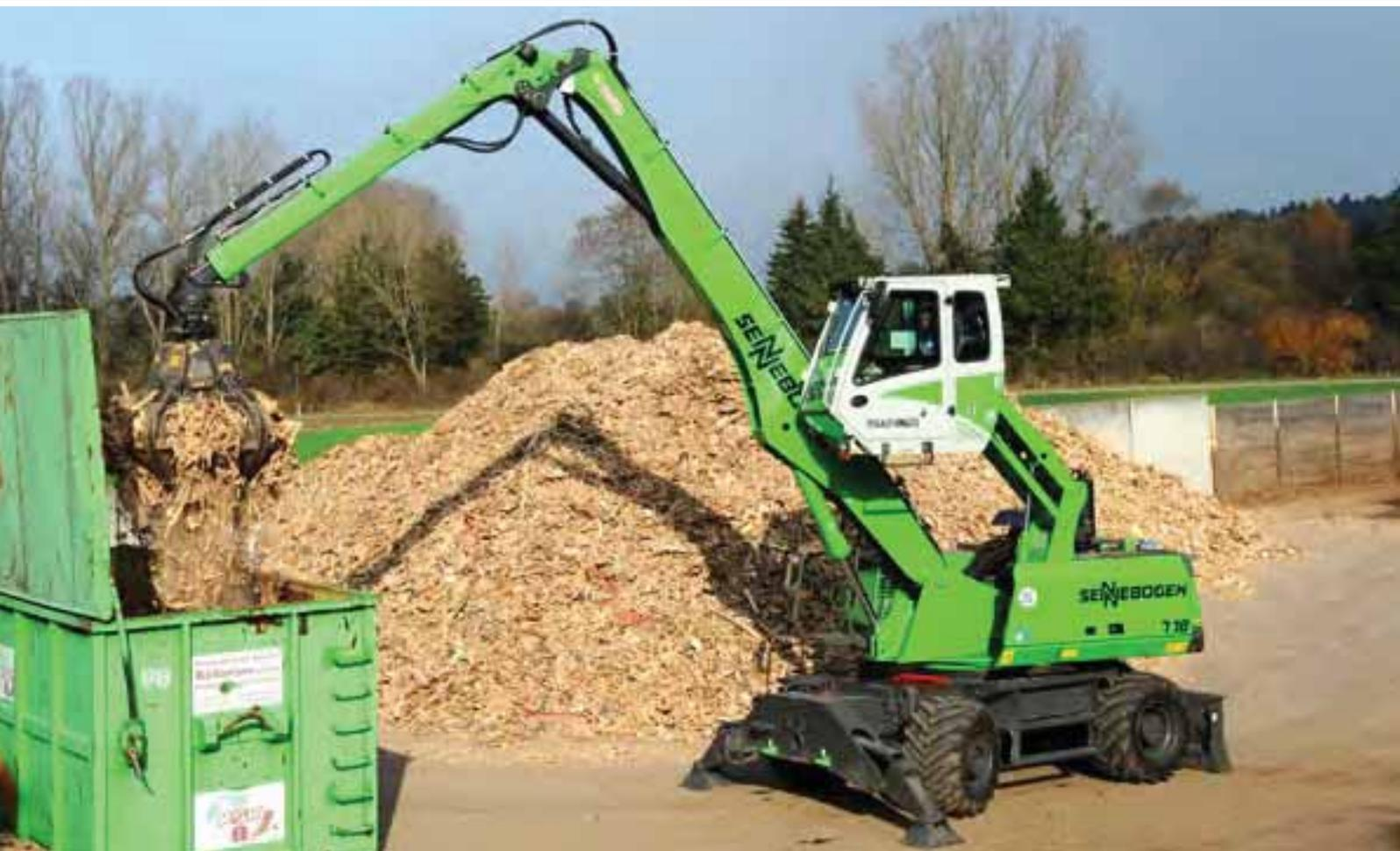
718 - with orange peel grab - loading a container with used wood; Germany
