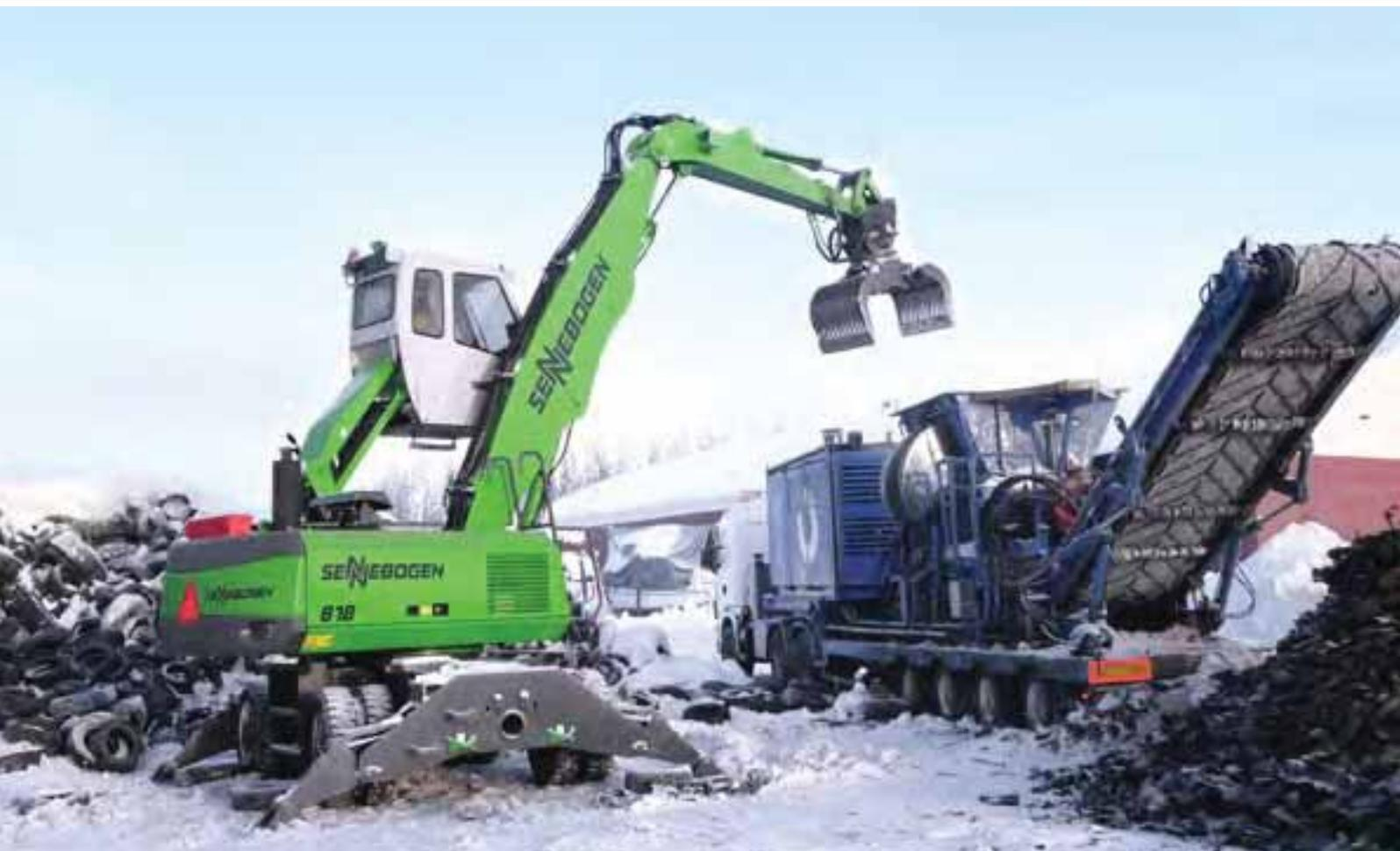
818 M – with sorting grab – feeding of a shredder with used tires; Finland
