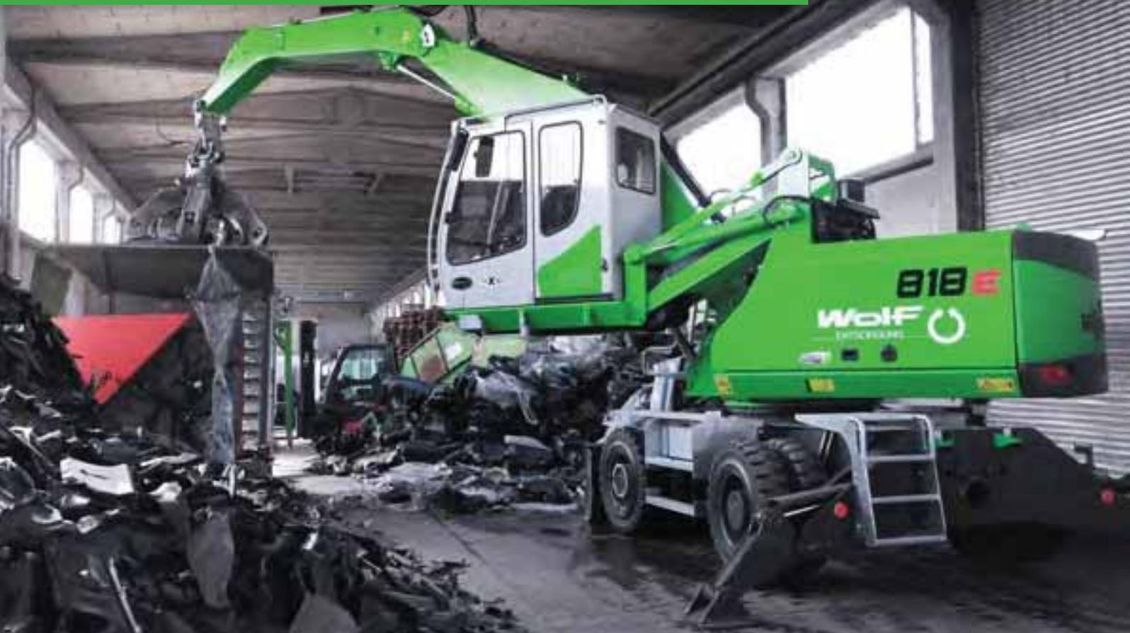
818 M – with orange peel grab – feeding a shredder with plastic inside a hall with low head room; Germany
