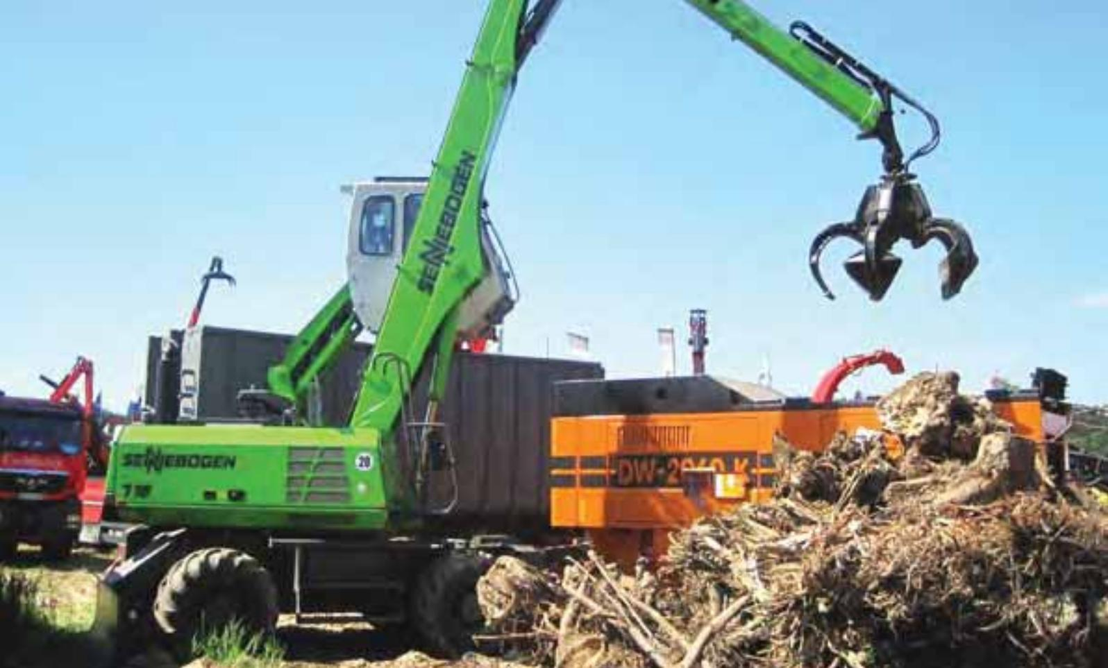
718 - with orange peel grab - feeding a shredder with used wood; Germany
