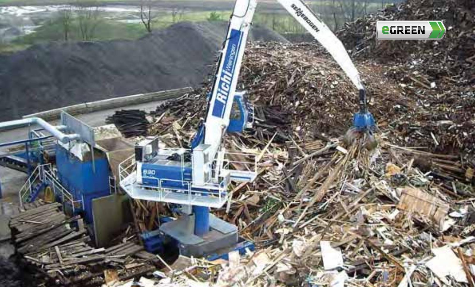
**830 Electro stationary – with orange peel grab – recycling of used wood; Switzerland**
