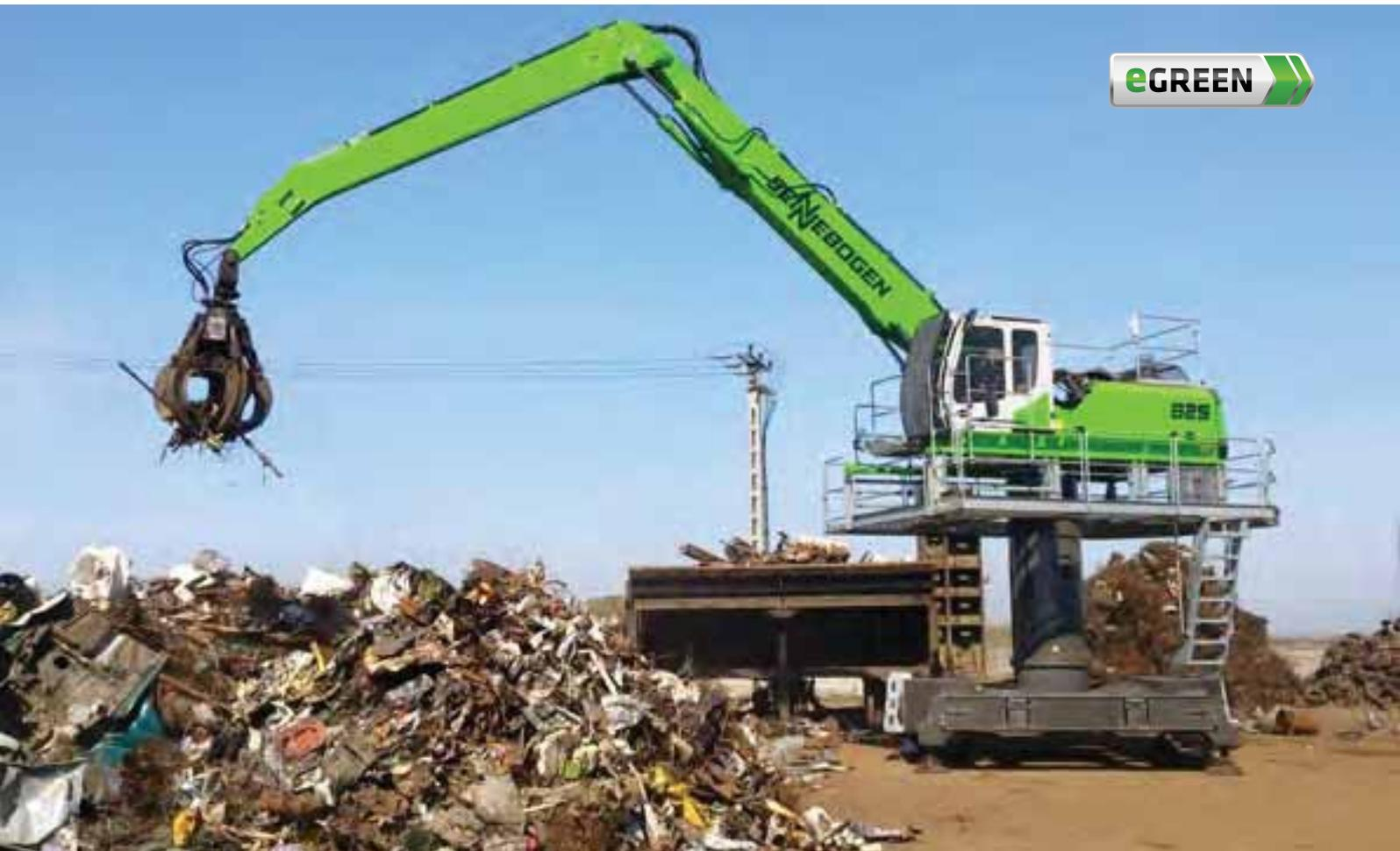
825 stationary Electro - with orange peel grab - feeding a scrap shear; Hungary
