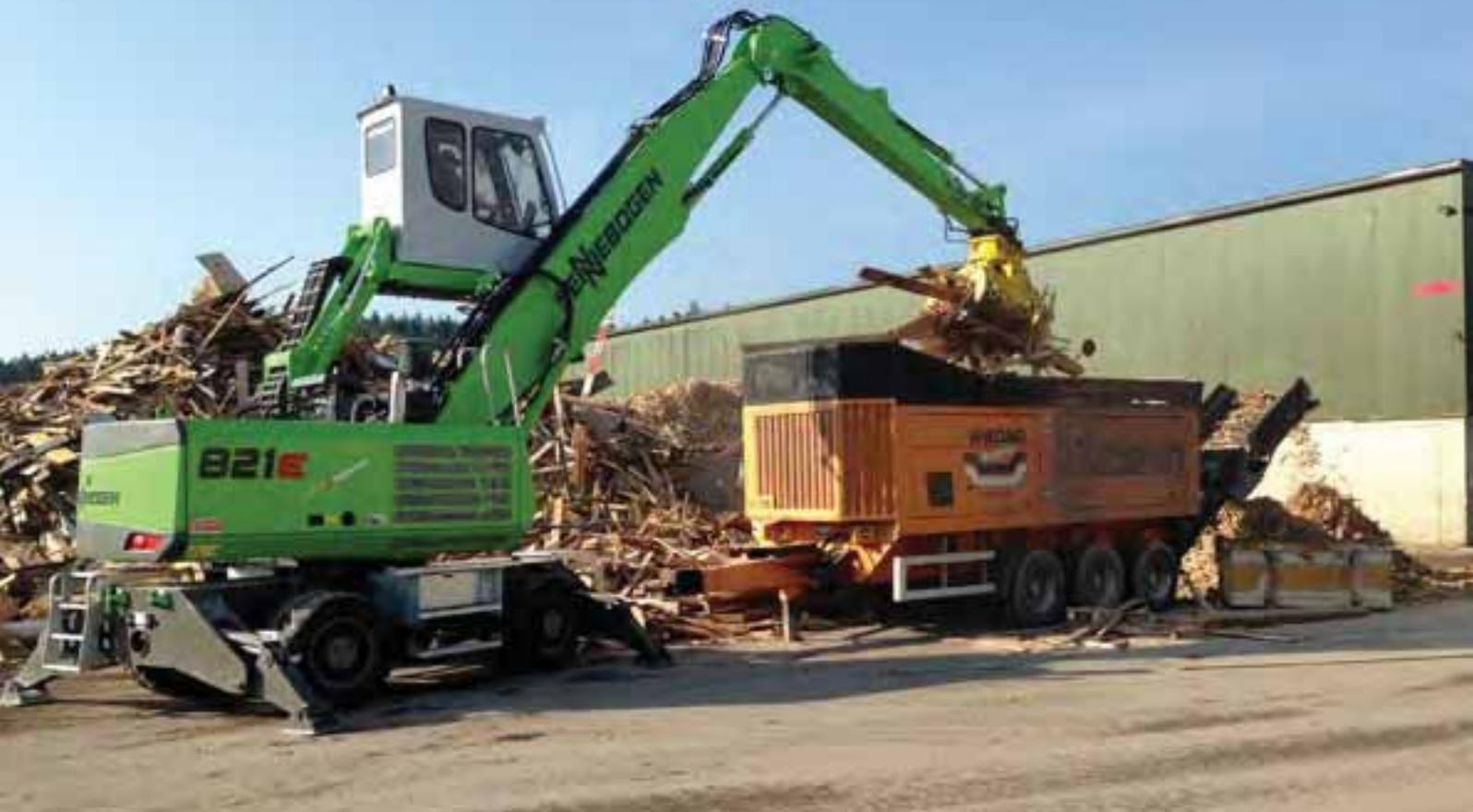
**821 M - with sorting grab - feeding a shredder with used wood; Switzerland**
