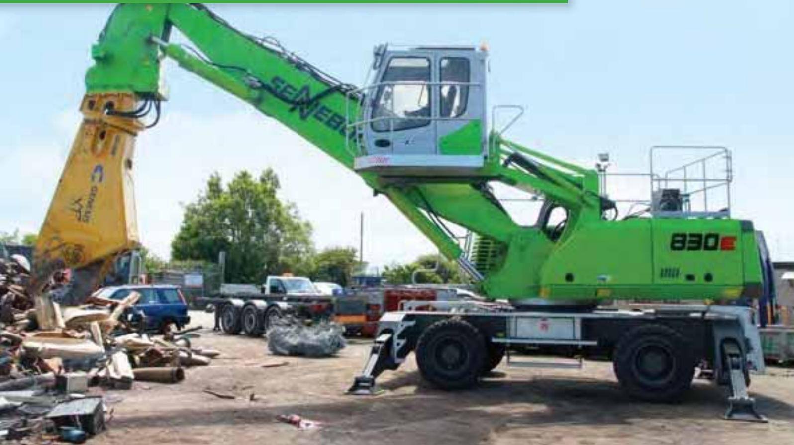
830 M Vario Tool - with 4 t scrap shear - shearing of scrap; Great Britain
