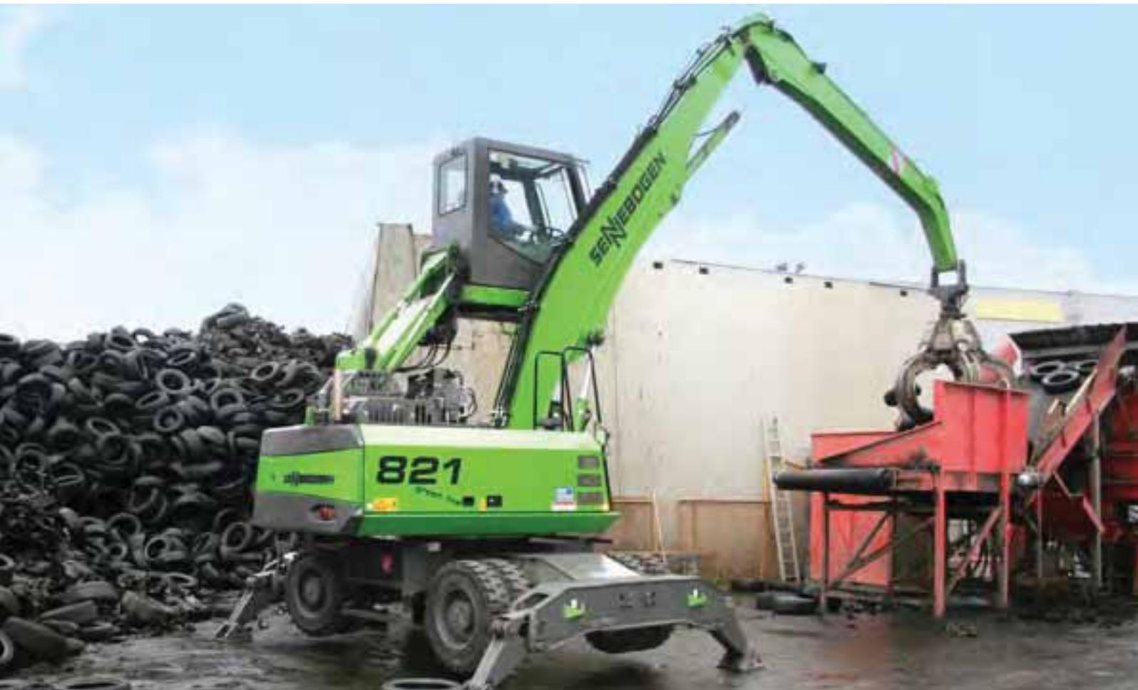
**821 M - with orange peel grab - feeding a shredder with used tires; Germany**
