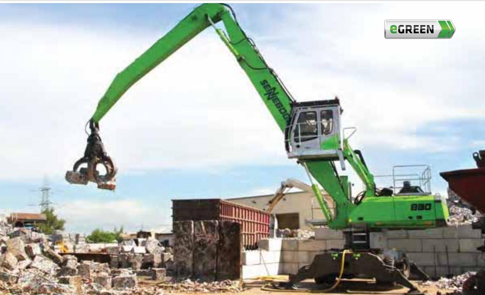
**830 M Electro – with orange peel grab – loading of steel balls; Great Britain**
