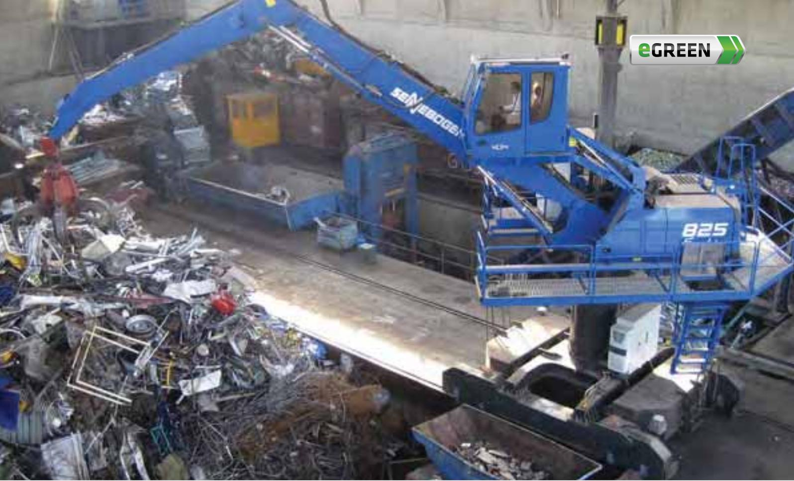
**825 Electro** - with rail undercarriage and orange peel grab grab - electrical feed from ceiling - feeding a scrap shear; Switzerland
