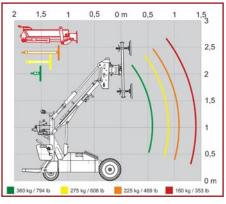
Lifting data with the different extention arms and with the front lift arm.
